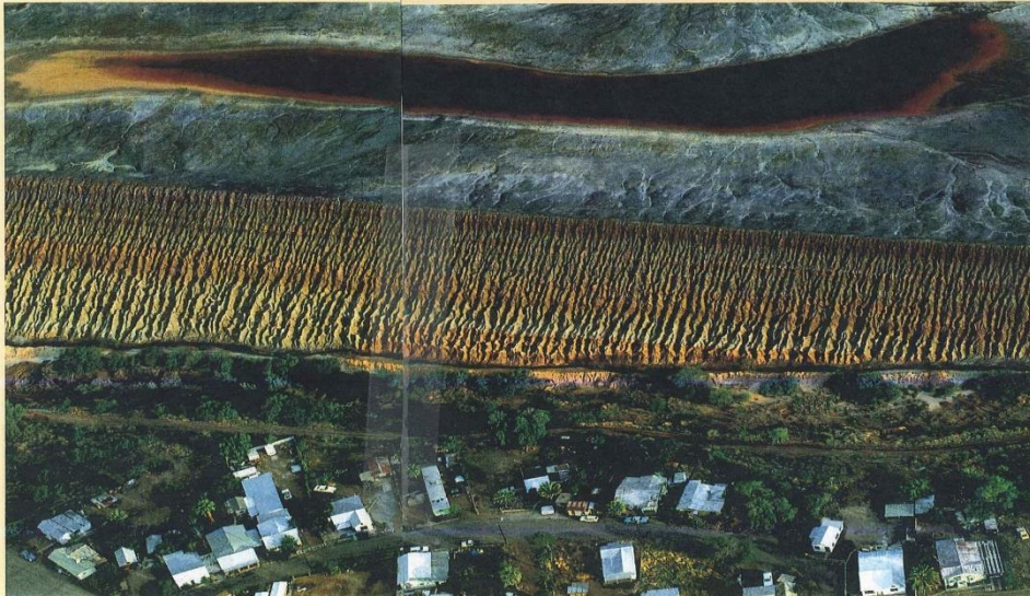
ARIZONA Backyard nightmare, a copper-tailings impoundment in Arizona reveals its toxicity in the sulfide-tinged rainwater pooling on its surface. Unless such piles of mining residue are properly contained, chemicals may leach freely into the groundwater.
